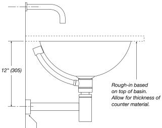
The compression fitting should not extend more than <sup>5</sup>/<sub>8</sub>" (16) beyond the finished wall in order to be covered by the Vitraform escutcheon.
