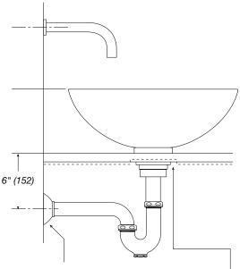
The compression fitting should not extend more than  $^{5}/_{8}$ " (16) beyond the finished wall in order to be covered by the Vitraform escutcheon.
