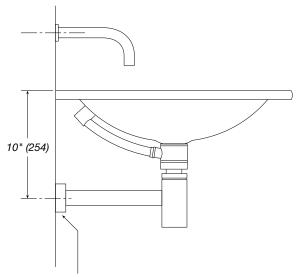
The compression fitting should not extend more than  $^5/_8$ " (16) beyond the finished wall in order to be covered by the Vitraform escutcheon.
