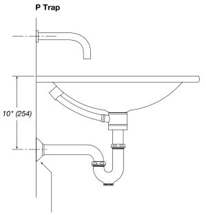
The compression fitting should not extend more than  $^{5}/_{8}$ " (16) beyond the finished wall in order to be covered by the Vitraform escutcheon.
